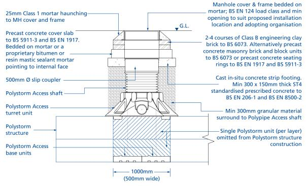
Please note: Above is a typical installation detail for a Polystorm tank with groundwater below the base of the unit. For installation with groundwater above the structure invert please contact our Technical Team on +44 (0) 1509 615100 or email civils@polypipe.com
