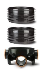
Polysewer Inspection Chambers are sold in component parts to be assembled on site. The base units are connected to Polysewer pipes, then side risers are used to build the chamber to the necessary height and can easily be cut to the correct level using a fine tooth saw. A seal ring is used to ensure a leak tight joint. Cover and frames are available in a range of load classifications.
