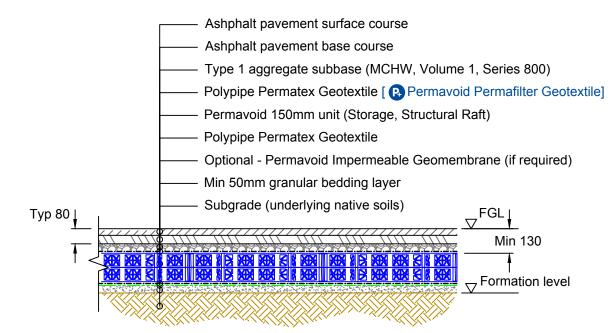
SEGREGATED CYCLE PATH - IMPERMEABLE SURFACE (Pedestrian Loading)
