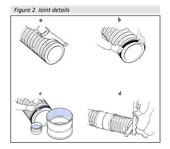
15.5 The pipe is offered to the socket, and is aligned and pushed fully home, as shown in Figure 2 (d).
